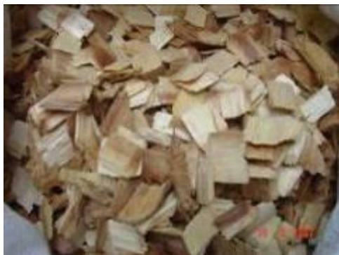
Wood chips after Chipper.
